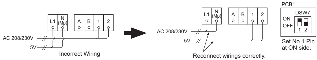
Fig. 8.1 Recovery from a Blown Fuse.
